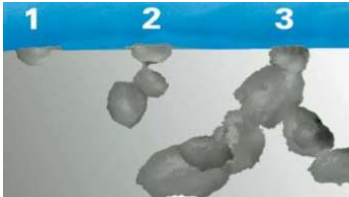
The stages of corrosion: 1. Initial Pit forms; 2. Auto catalytic process speeds up as concentrated solution becomes more aggressive; 3. Leak occurs as pit breaks through outer surface.
