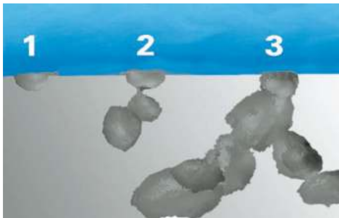
The stages of corrosion: 1. Initial Pit forms; 2. Auto catalytic process speeds up as concentrated solution becomes more aggressive; 3. Leak occurs as pit breaks through outer surface.
